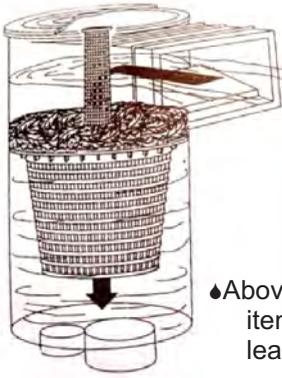
The patented\* Vented Skimmer Basket solves three potentially serious problems for the swimming pool owner by providing an above water handle that also serves to prevent skimmer blockage caused by a full basket of debris.
